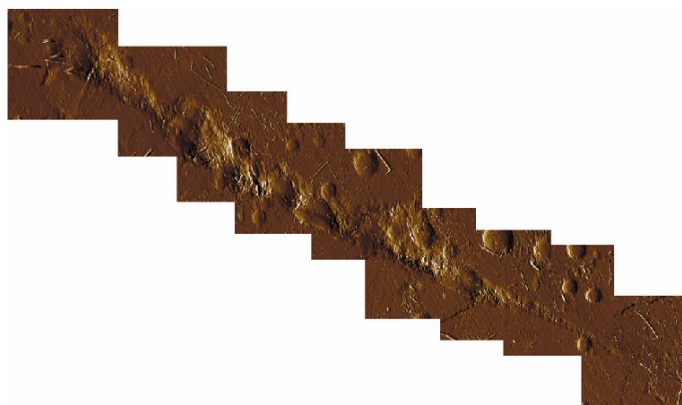
Figure A 125-micrometer-long etch channel produced by fungus Talaromyces flavus on the surface of iron-bearing mineral lizardite. Credit: Zibo Li
